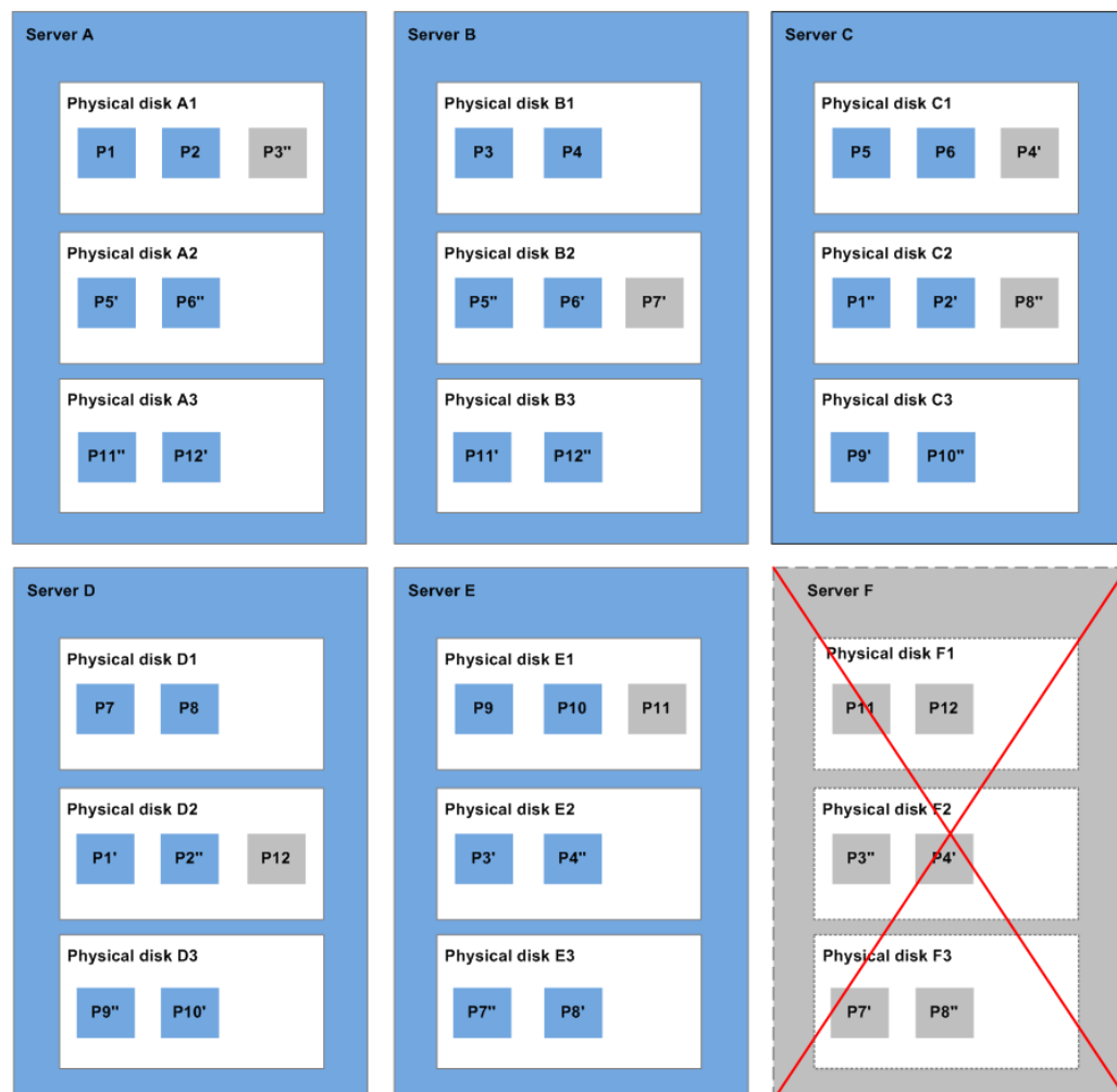
Figure 6-3 Data rebuild principle
